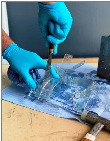
Step 3: Gently pull off the supports and get rid of the bigger parts e.g. with isopropanol as a primary cleaning if needed. It is important to get rid of all these parts to protect the RS wash
