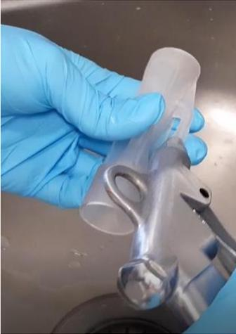
Step 4: **Check** the VENTURI NOZZLE for residual resin (especially in the critical thin parts). **Very important: After cleaning, there must be no residual material on the object!**
