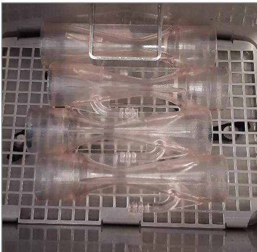
Step 1: After finishing the print job, please remove the VENTURI NOZZLE carefully from the build platform.
